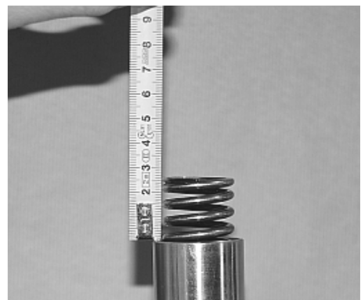
7B: MEASURE DISTANCE (CASE SPRING OUTSIDE)
