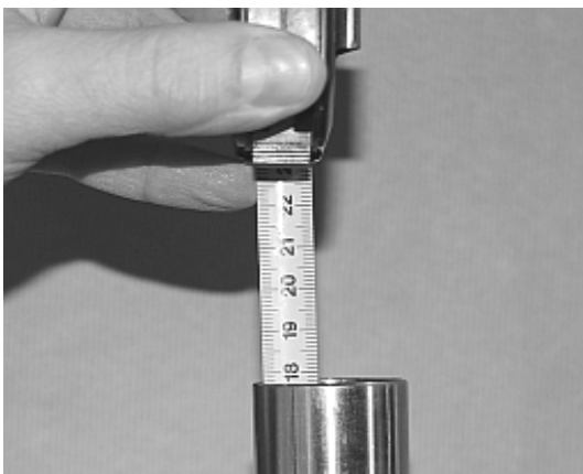
7a: MEASURE DISTANCE (CASE SPRING INSIDE)
